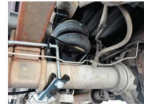
Aftermarket/Secondary Air Suspension (Air Bag Supplements the Primary Leaf Spring Assembly)
