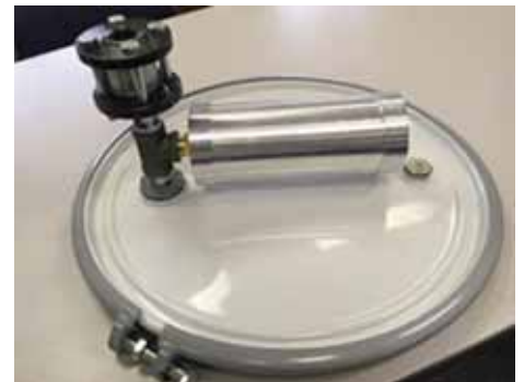
This HEPA filtration system was installed on the lids of the RNS drums.
