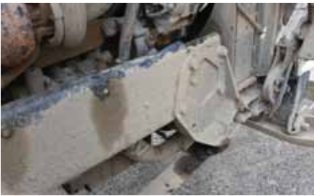
Missing auxiliary steering box. Photos by Ofr. Michael Kasprzak. Cassiar Junction Weigh Station, Yukon, Canada.
