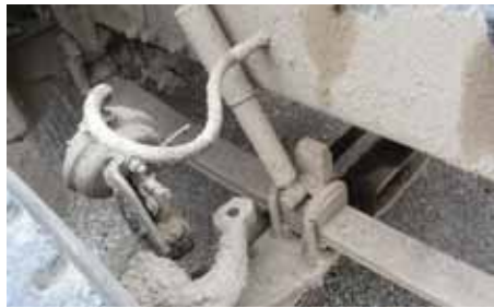
Missing auxiliary steering box. Photos by Ofr. Michael Kasprzak. Cassiar Junction Weigh Station, Yukon, Canada.
