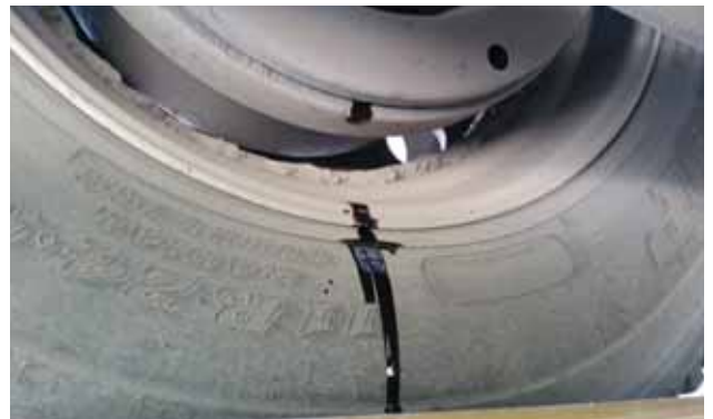
Leaking wheel seal. Photo by Ofr. Michael Kasprzak and Ofr. Sebastien Nadeau. Whitehorse Weigh Station, Yukon, Canada.
