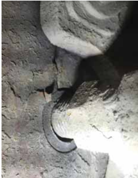
Cracked brake chamber. Photo by Ofr. Brett Barteaux. Whitehorse Weigh Station, Yukon, Canada.
