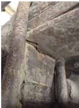
Broken main leaf (spring). Photo by Ofr. Sheldon Barteaux. Whitehorse Weigh Station, Yukon, Canada.
