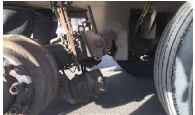
Broken axle mount on a trailer. All tires and wheels were removed from the axle. Photo by Ofr. Sheldon Barteaux. Whitehorse Weigh Station, Yukon, Canada.
