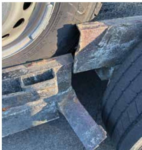
Broken trailer frame rail – driver side.
