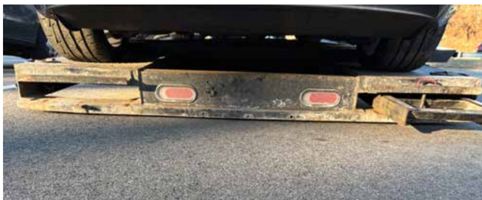
Insufficient road clearance – rear of trailer.
