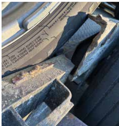
Broken trailer frame rail – front view.
