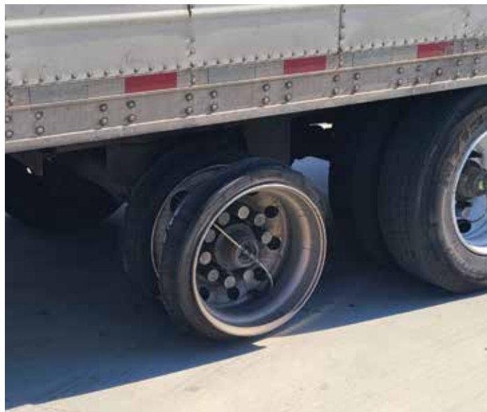
A completely blown-out tire; X-5 on the right side of the trailer.
