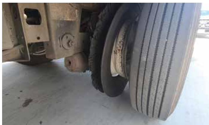
A tire that is a bit more than just flat; X-4 on the left side of the trailer.
