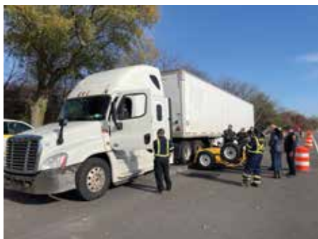
The New York State Department of Transportation, a participating jurisdiction in SafeDRIVE, operates a performance-based brake tester as part of this enforcement wave.
