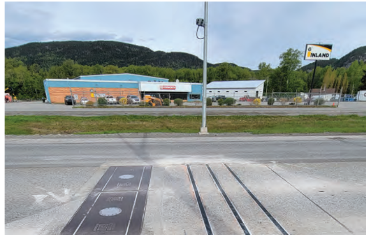
The Terrace, British Columbia, single load cell WIM scale and tire anomaly and classification system.
