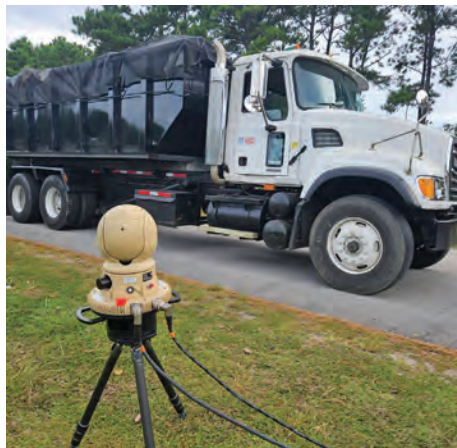
NCSHP utilized a forward-looking infrared thermal camera to check brake temperature.
