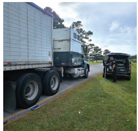
Over a four-day span, a total of 70 CMVs were weighed with the portable scales and WIM technology.
