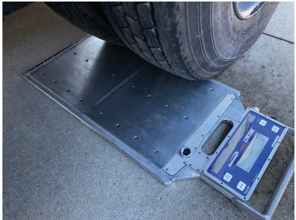
The Dual Wheel Load Scale measures individual tire loading, enabling inspectors to identify overrated tires.
