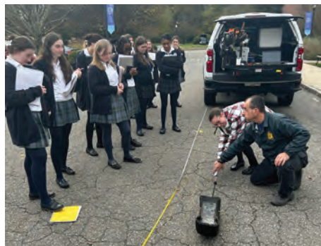
Students complete the field exercise by measuring skid marks and determining the coefficient of friction on the roadway.
