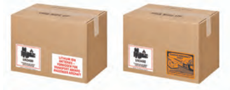
Lithium batteries shipped under the exception in § 173.185(c) displaying the lithium battery mark and the appropriate aviation warning.
