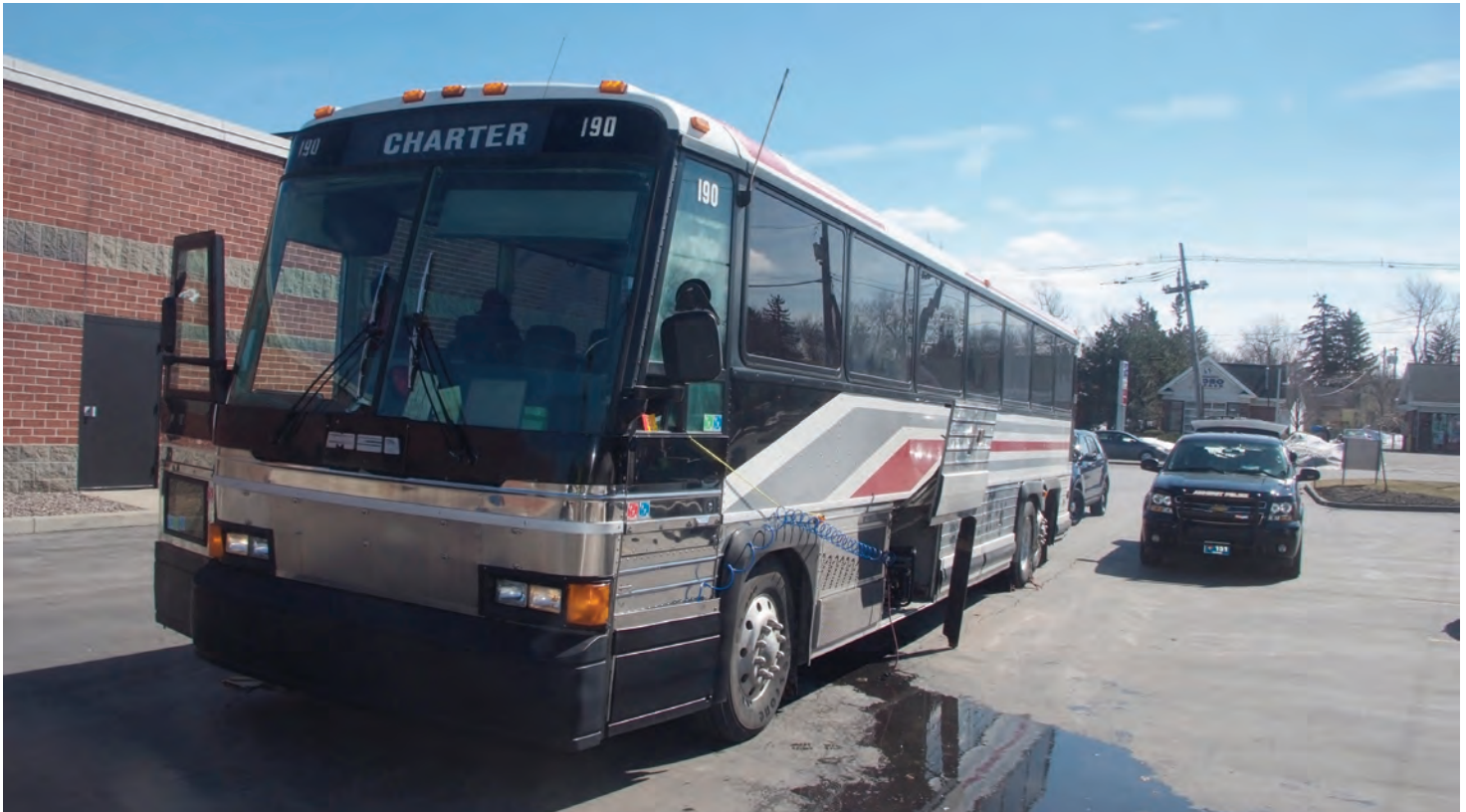
PICTURE #1: Bus pulled over by Ofc. Murphy, who found multiple violations. Look at the coiled line screaming, "Here I am! Pull me over!"
