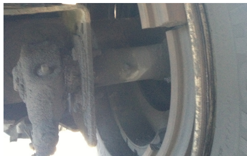
Broken Drum. OOSC, Part II, g.(4) / 393.47(a)-U.S.
