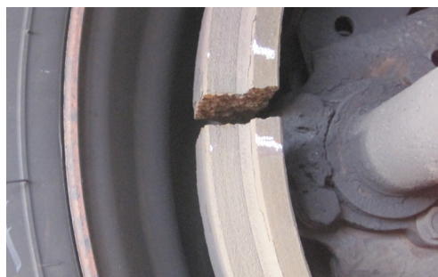
Broken Drum. OOSC, Part II, g.(1) / 393.47(a)-U.S.
