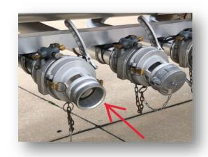
The discharge pipe dust/safety cap is not a stop-valve or other leak-tight closure at the end of the discharge pipe. The dust/safety cap is a convenience to the driver/carrier as its intention is to keep debris and other contaminates out of the discharge line connection area.
