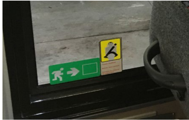
Green pictograph indicating an exit is located to the front of this occupant's space.
