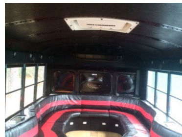
This converted school bus no longer meets Method Two Option A due to the removal of the rear exit door. A roof hatch has been added to comply with Method One.
