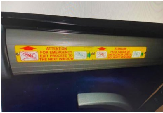
Pictograph and text clearly indicating this non-opening window is not an emergency exit and the location where the exit may be found.
