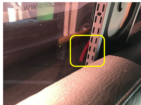
Custom panel and seat back blocking the release mechanism, making the exit inoperative.
