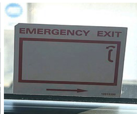
This same marking would be acceptable when found in the occupant space of an emergency window with a single release mechanism to the right.
