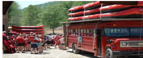
Providing transportation to adults will reduce the manufacturer's pupil seating capacity from three to two per seating surface. This bus does not require a roof hatch if the seating capacity is under 63 for Option A or under 75 for Option B.
