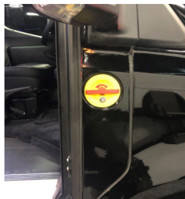
Exterior door release valve at the entrance door of a custom limousine.
