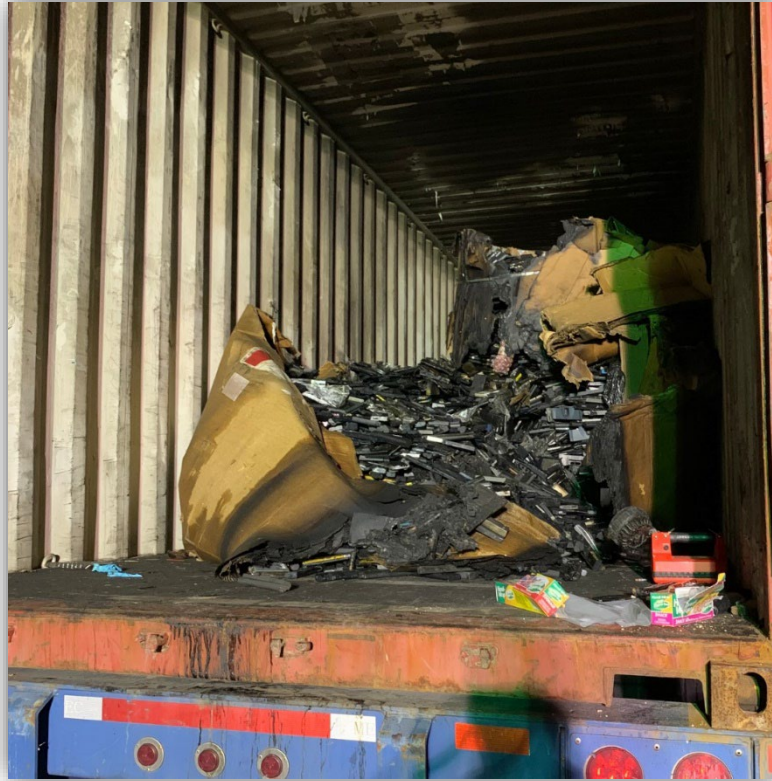
Aftermath of a fire in an undeclared lithium battery shipment
