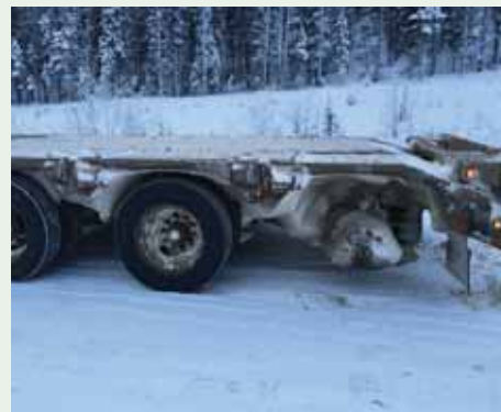
Missing trailer wheels. Photo by Ofr. Carol Bates, Whitehorse Weigh Station, Yukon.
