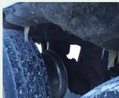
Missing tire. Photo by Ofr Sheldon Barteaux, Whitehorse Weigh Station, Yukon.
