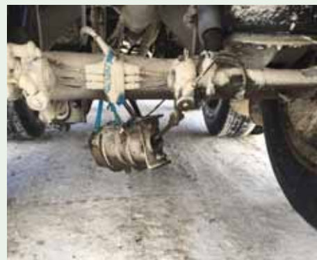
Brake chamber improperly attached to an empty fuel truck. Photo by Ofr. Sheldon Barteaux, Whitehorse Weigh Station, Yukon.
