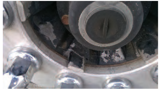
Cracked on the left front steering axle. Note the circumferential crack across the flanges for the hub piloted wheel. Photo by Philip Zeman, Transportation Inspector. Anthony Port Of Entry, I-10 Westbound, New Mexico.
