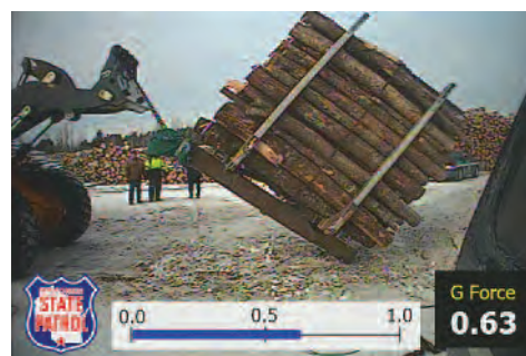
Image 8: Screen capture from the VBOX video showing a load of hardwood with a single 5/16" grade 70 transport chain. The current force experienced by the load is 0.63 g, which is obtained at an angle of approximately 39 degrees.
