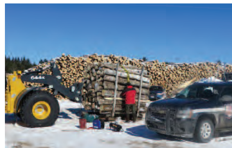
Image 7: A single strap is secured over a bunk containing low-friction logs.
