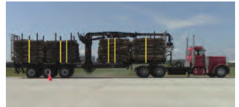
Image 4: Past enforcement practice would require this trailer with a center-mounted crane to have two tie-downs on the center stacks and one tie-down on the end stacks as drawn because the vehicle does not technically meet the specific definition of a crib-type vehicle.
