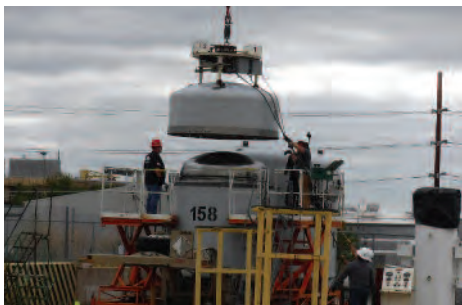
TRUPACT II outer cover is removed.
