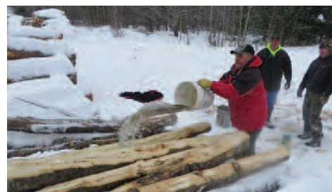
Image 6: Author Capt. Brian Ausloos prepares low-friction logs with water after peeling.
