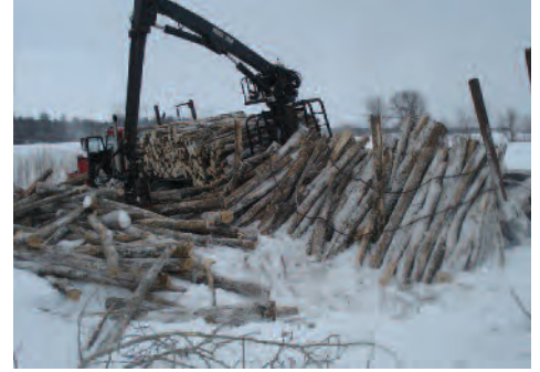
Image 3: Log spill in Wisconsin. Logs loaded crosswise on a frame vehicle are secured with two longitudinal tie-downs.
