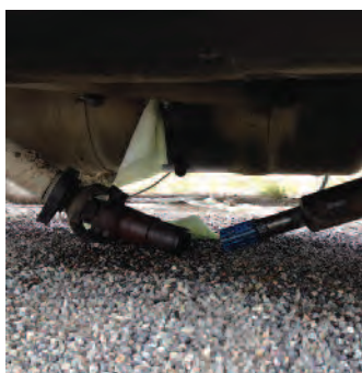
The vehicle experienced driveshaft failure in front of the Whitehorse Weigh Station and the driveshaft punctured the fuel tank. Photo by Officer Sheldon Barteaux, Whitehorse Weigh Station, Yukon.
