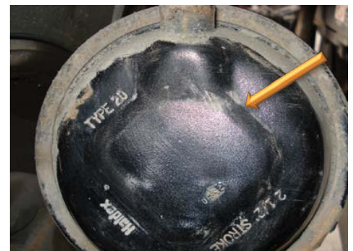
Examples of square-shapes embossed into chamber pressure caps.
