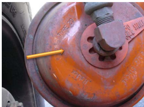
Examples of square-shapes embossed into chamber pressure caps.
